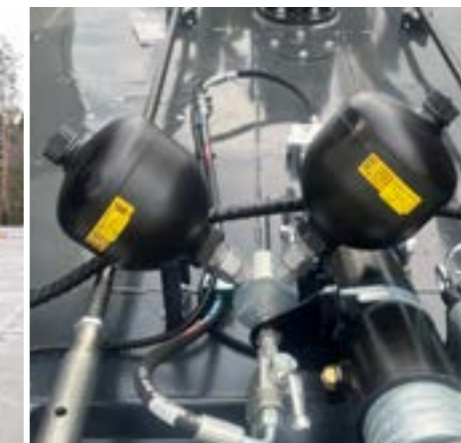
hydroaccumulators are used with amortized suspension (option)
